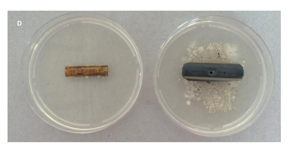
Photo D compares the filters from the dripper lines. The Rainmaker treated filter on the left showed hardly any bacterial film growth compared to the untreated filter on the right.
